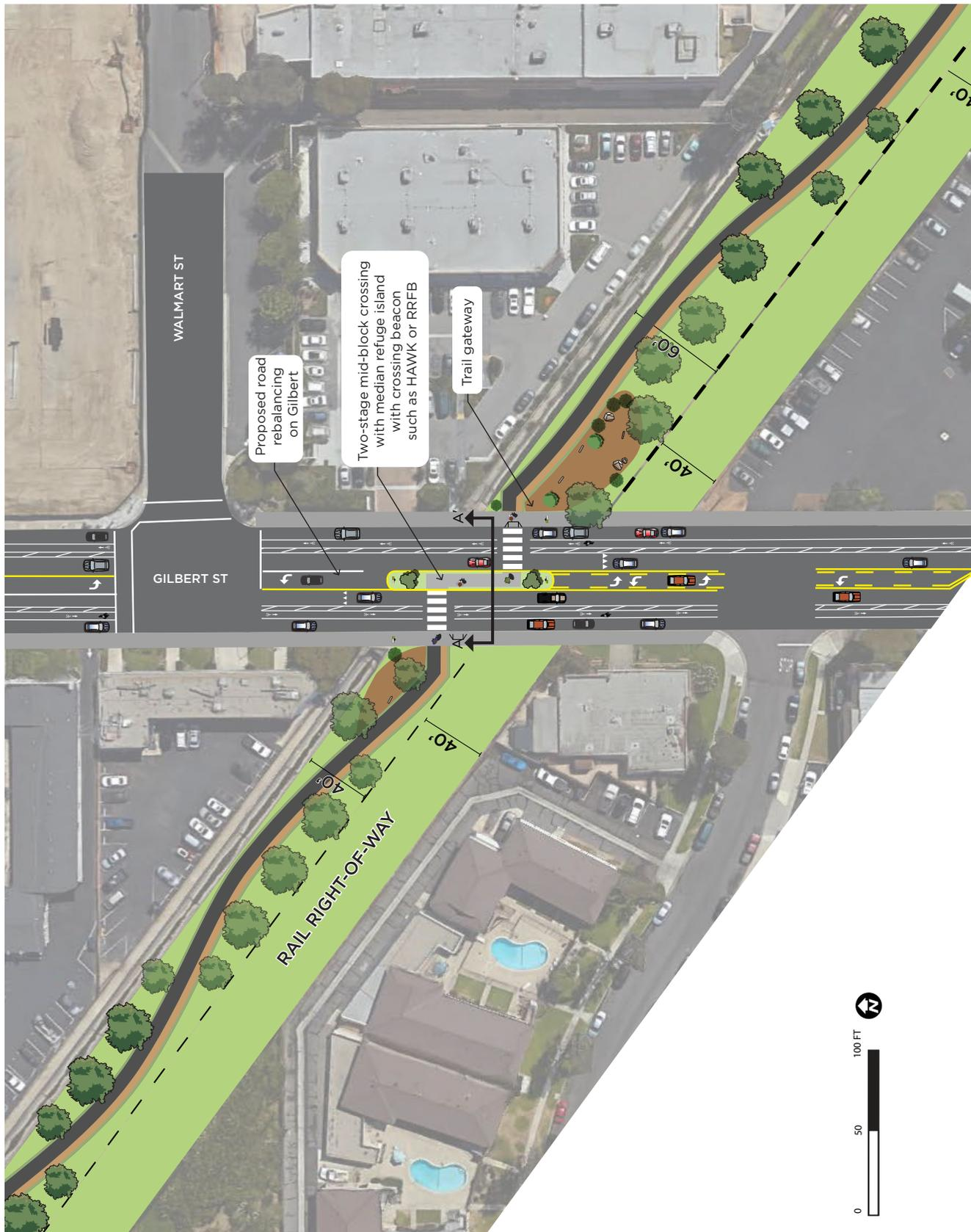
Figure 8-6: Existing condition and conceptual rendering of the PE ROW Trail crossing at Gilbert Street
