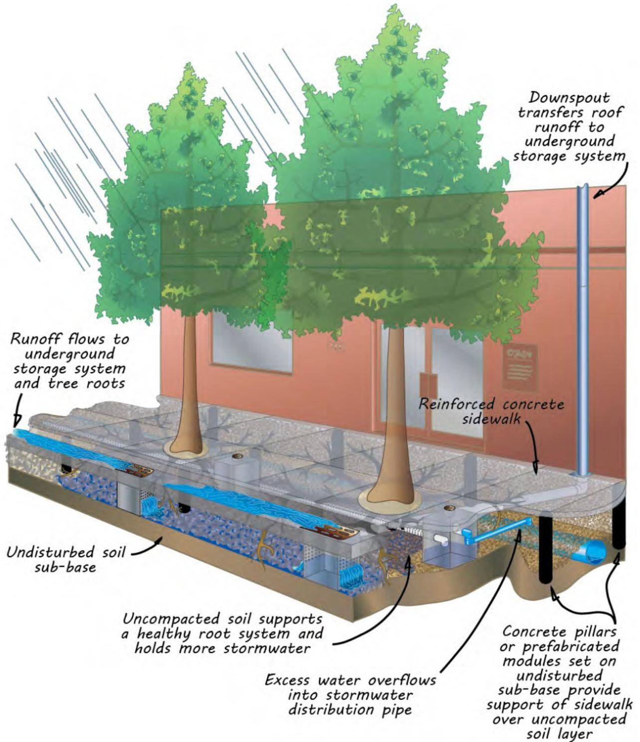
**Above:** Suspended sidewalks use pillars or structured cell systems to support reinforced concrete, increasing the volume of uncompacted soil in subsurface planting areas and enhancing both root growth and stormwater storage.
