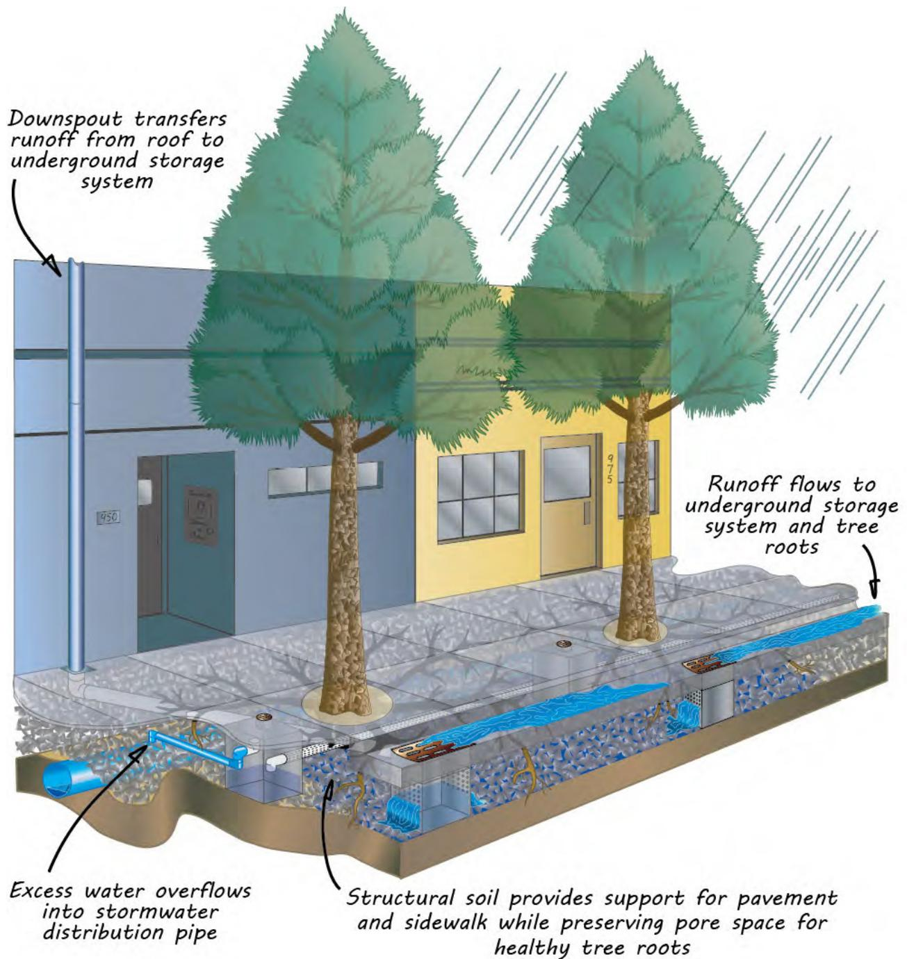
**Above:** Structural soil is a highly porous, engineered aggregate mix, designed for use under asphalt and concrete as a load-bearing and leveling layer. The created spaces allow for water infiltration and storage, in addition to root growth.
