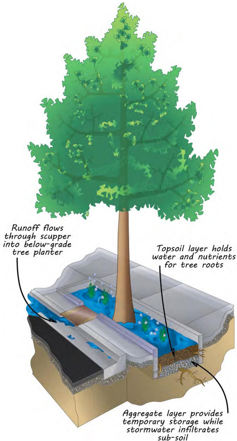
**Above:** Stormwater tree pits are designed to collect runoff from streets, parking lots, and other impervious areas. Stormwater is directed into scuppers that flow into below-grade planters that then allow stormwater to infiltrate soils to supplement irrigation.
