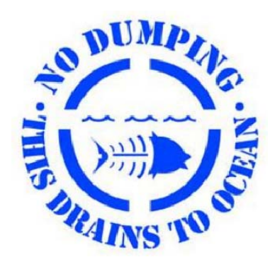
1 CATCH BASIN STENCIL DETAIL
