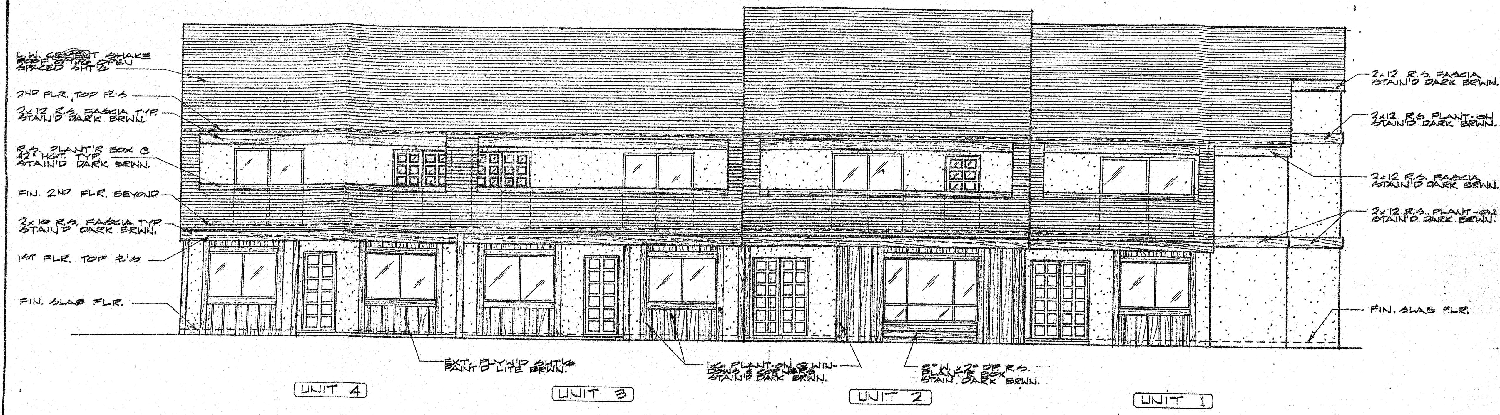
EAST OR FRONT ELEVATION - BUILDING "A" SCALE: 1/4" = 1'-0"
