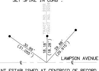
POINT ESTABLISHED AT CENTROID OF RECORD TIE DISTANCES. MEASURED DISTANCES ARE TO ESTABLISHED POINT.
