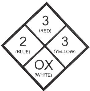
Through this system, Fire Fighters can tell at a glance the worst case hazard levels that can be found within the building. This can be of great assistance in an emergency!
